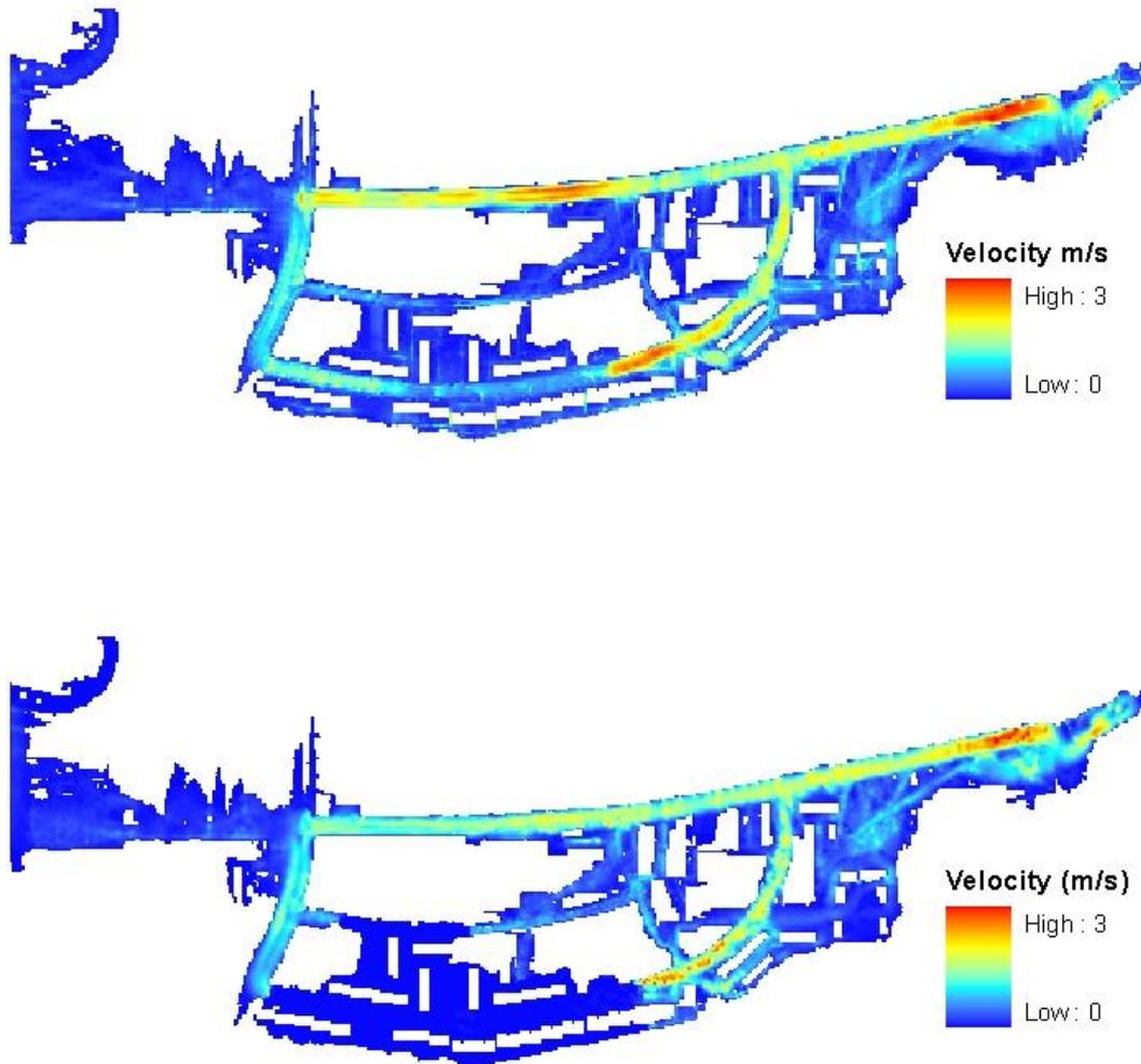
Figure 3. Maximum velocity grids. Upper panel: JFLOW SWE scheme. Lower panel: TUFLOW.
