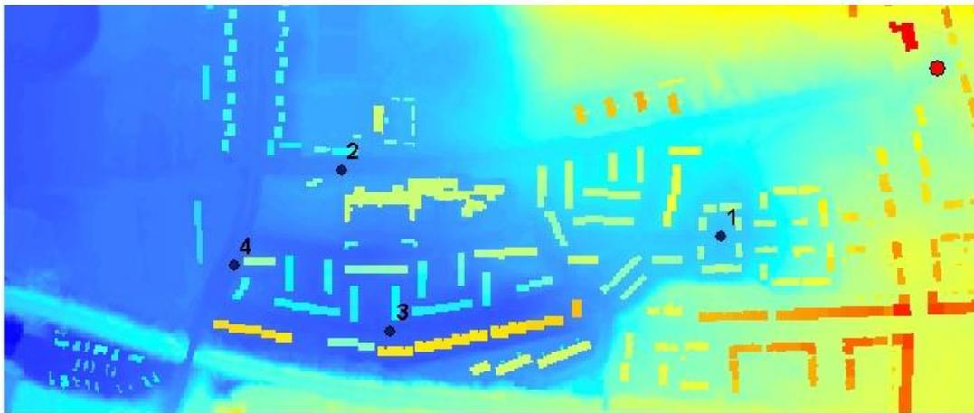
Figure 1. Glasgow urban test case DEM showing numbered monitor point locations and inflow location (red dot in upper right of the image).
