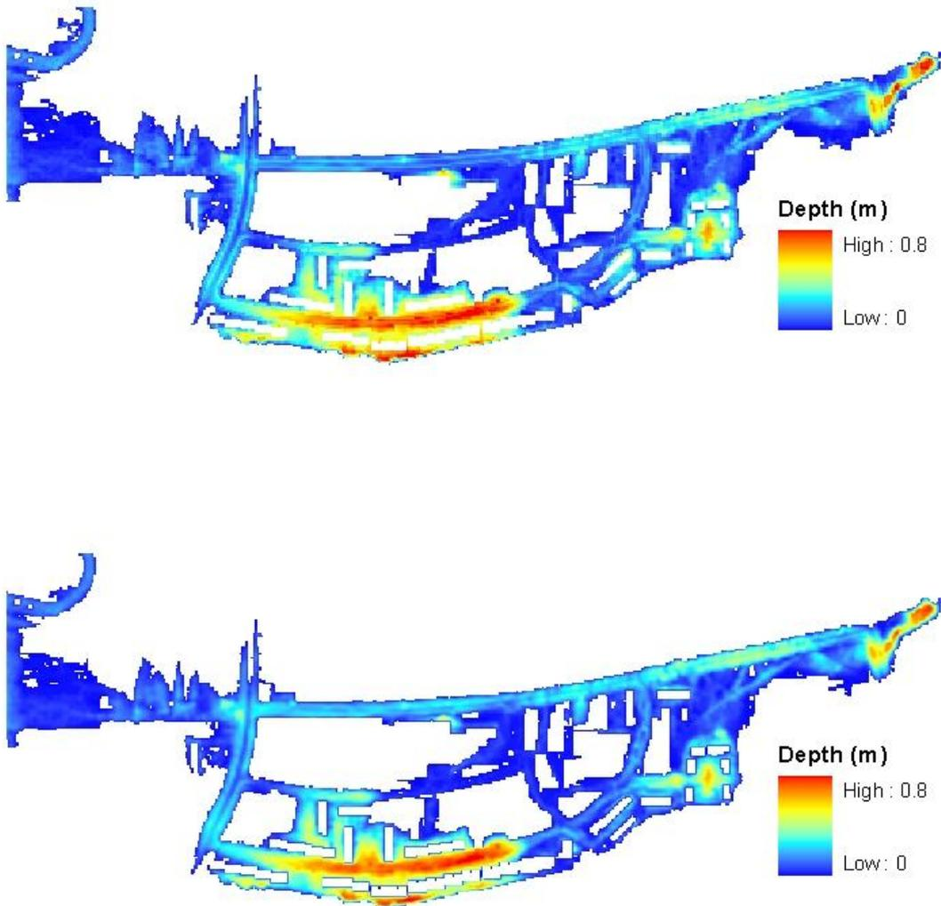
Figure 2. Maximum depth grids. Upper panel: JFLOW SWE scheme. Lower panel: TUFLOW.
